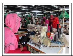
NC Photo-1: Eye Guard Displaced (Overlock m/c)
