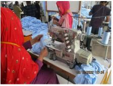
NC Photo-2: Eye Guard Displaced (Flatlock m/c)
